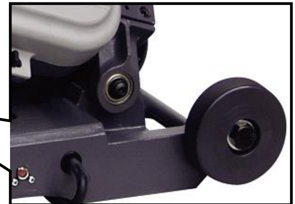
Smooth movement of frame with ball bearings.
