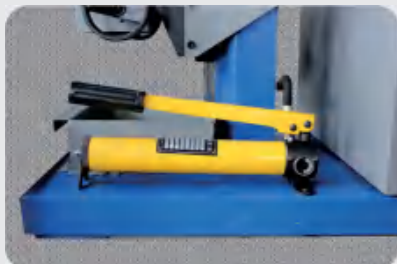
液压调高 Hydraulic height adjustment
