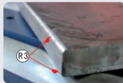
坡口加工后 After processing
