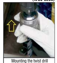
Mounting the twist drill
