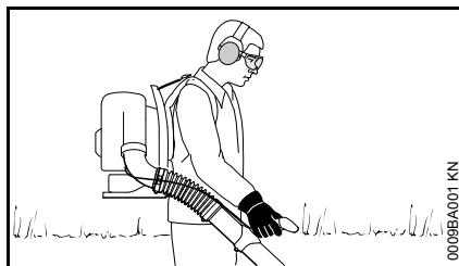
The machine is carried as a backpack. Hold and control the blower tube with your right hand on the control handle.
