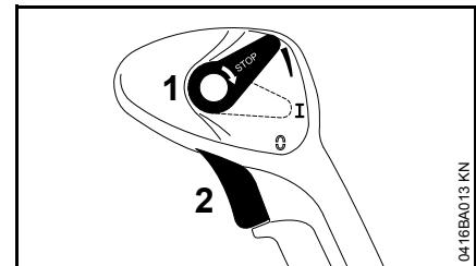
The throttle trigger (2) can be locked in any position.
